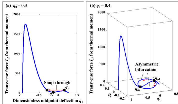
Fig. 3. Bifurcation diagram of FGM microbeam actuated by thermal loading.
