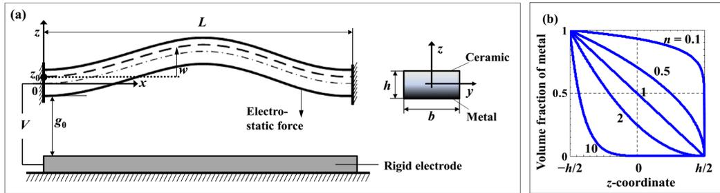
Fig. 1. (a) Initially curved functionally graded material microbeam under distributed electrostatic force (direction indicated by arrow). (b) Variation of volume fraction of metal along beam thickness at different levels of power law index  $n$ .
