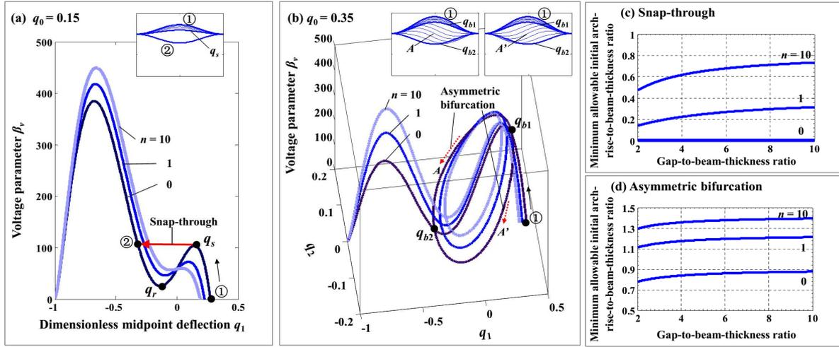
Fig. 2. (a), (b) Bifurcation diagram of FGM microbeam actuated by electrical loading. (c), (d) Minimum allowable ratio between the initial arch rise and the beam thickness for the existence of snap-through and asymmetric bifurcation.
