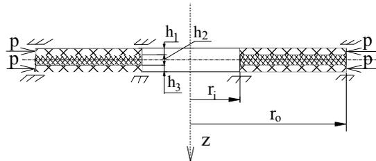
Figure 1. Scheme of three-layered annular plates with composite facings.
