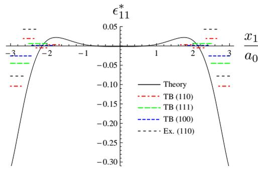
**Figure 2.** Surface relaxation delineated by strain component,  $\epsilon_{11}^*$  versus normalized coordinate  $x_1/a_0$  for Ag film of thickness  $6a_0$ , where  $a_0$  is the lattice parameter. The available values of the average strain computed via tight-binding scheme [1] as well as the experimental data [2] are plotted for comparison.
