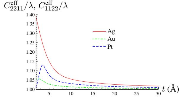
**Figure 3.** The normalized components of the effective elastic constants,  $C_{2211}^{\text{eff}} = C_{2211}^{\text{eff}}$  with respect to Lamé constant,  $\lambda$  versus film thickness in units of  $\text{\AA}$  for Ag, Au, and Pt.
