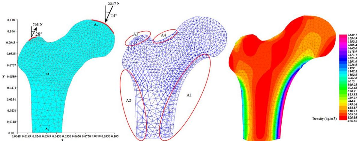
Figure 1: Simulations of internal and external bone growth at the macroscopic level. (a) Loading conditions and original structure with uniform distribution at the beginning of simulation: initial density= 800 kg/m<sup>3</sup>, (b) Bone density distribution after 140 growth-timesteps, (c) Overlay plots of the original bone and grown bone meshes
