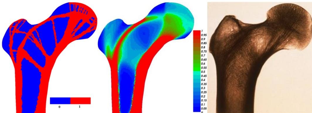
Figure 2. Optimum internal architecture of the femoral head using SIMP approach (left) and homogenization (middle). Right view: Roentgenogram of the internal structure of the femur (Tobin, 1955). Load is shown in figure 1a.
