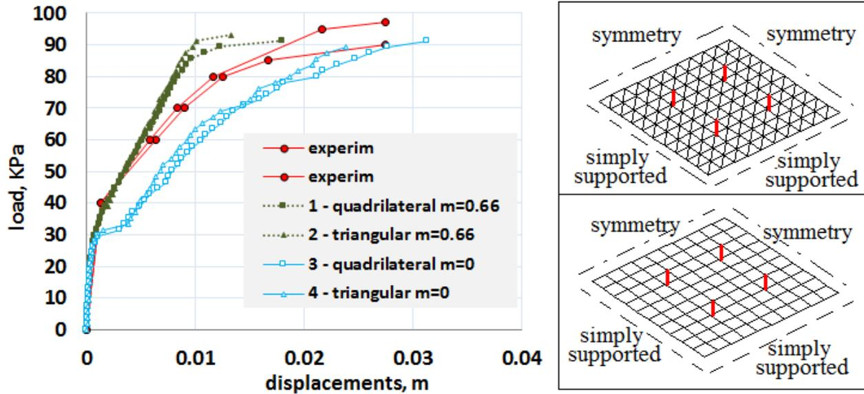
Fig. 1 Load-displacement diagram and finite element meshes
