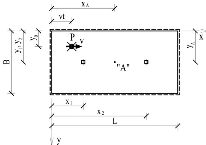
Fig 1. Rectangular thin plate simply supported on all edges with two point supports, subjected to a moving force
