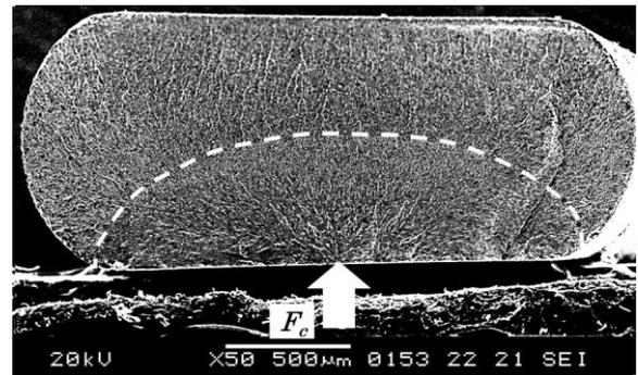
Fig. 2 SEM photograph of fracture surface of as-received tape for  $\epsilon_a = 1.26\%$  and  $N_f = 5906$
