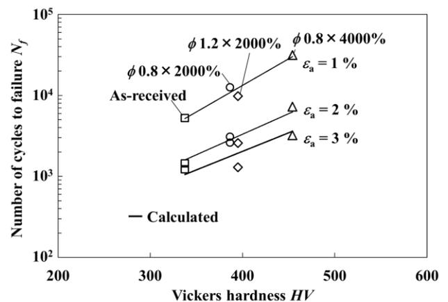
Fig. 4 Relationship between number of cycles to failure and Vickers hardness for various strain amplitudes  $\epsilon_a$
