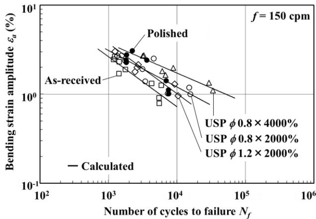
Fig. 1 Relationship between bending strain amplitude and the number of cycles to failure
