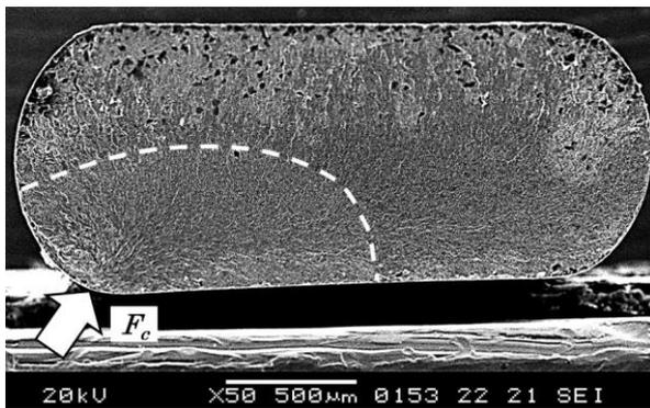
Fig. 3 SEM photograph of fracture surface of USP-treated tape for  $\epsilon_a = 1.68\%$  and  $N_f = 6788$
