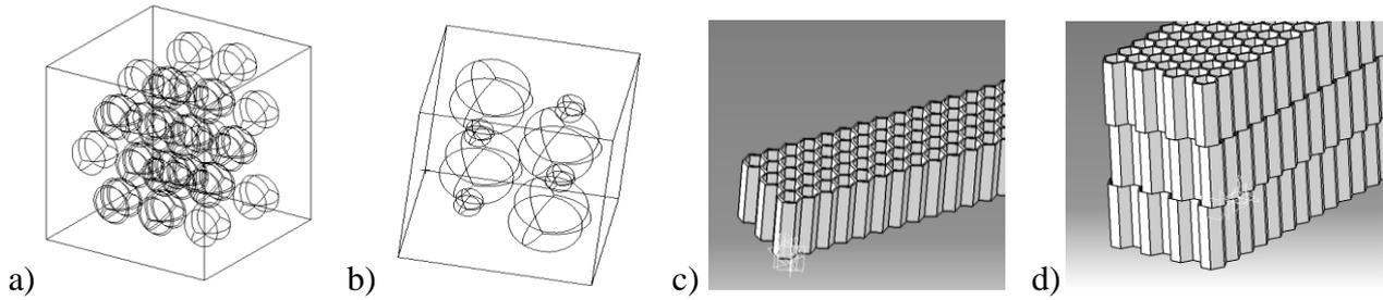
Fig. 1. RVE models regular (a), irregular (b) and parametric models consist of one layer (c) and three layers (d).
