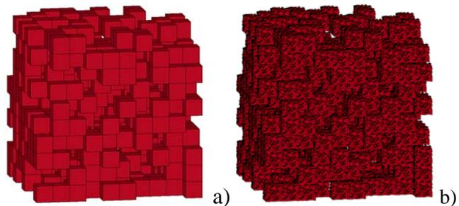
Figure 2. Example of the numerical model used in research – model was developed with the use of linear randomization,  $p_0=0.6$ : a) first porosity level, b) second porosity level.
