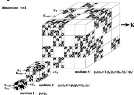
Figure 1. Schematic representation of the hierarchical (fractal) model of a porous medium. The dimension is  $n = 4$ . The basic porosity is  $p_0 = 0.5$  [5].
