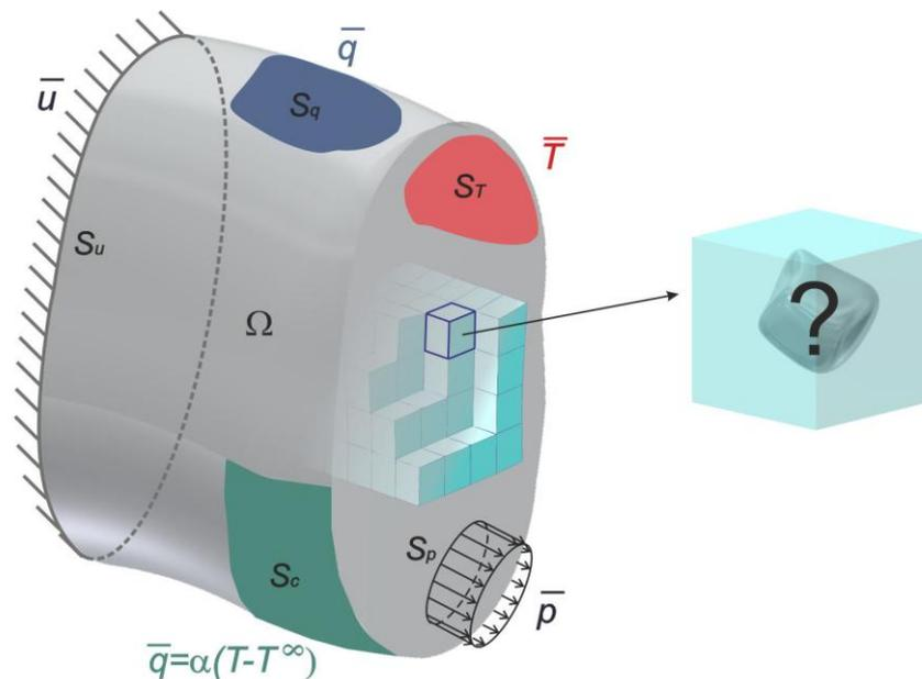
Figure 1. Two-scale model of the 3D porous body under thermal and mechanical loads
