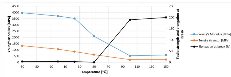
Figure 1. Temperature dependence of mechanical strength.
