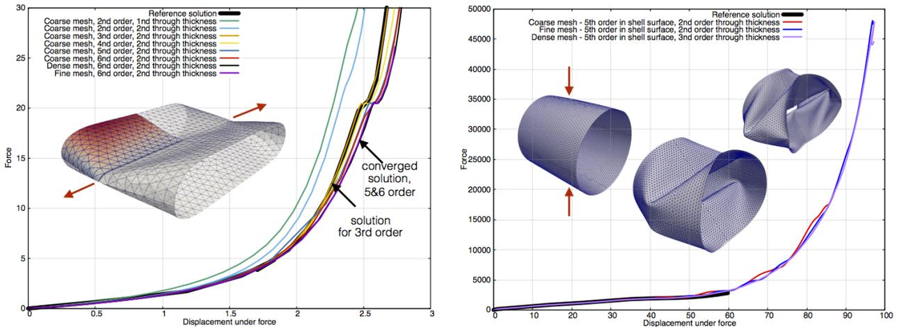
**Figure 1.** Pinched cylinder without diaphragm tension on the left and with diaphragm compression on the right. See [4] for more information about geometry, material parameters and reference solution. Analysed meshes are available from [1].
