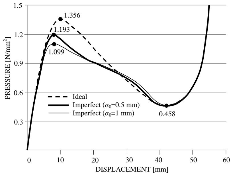
Fig. 2. Fundamental load-displacement path for apex node
