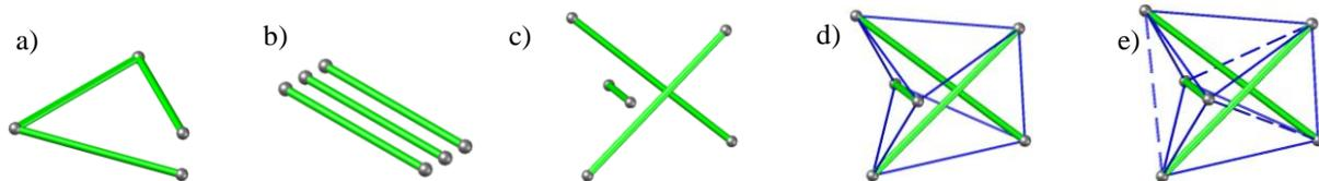
Fig. 1. A tensegrity configuration and tensegrity system: a) and b) not a tensegrity configuration, c) the tensegrity configuration, d) the minimal tensegrity system, e) the non-minimal tensegrity system.
