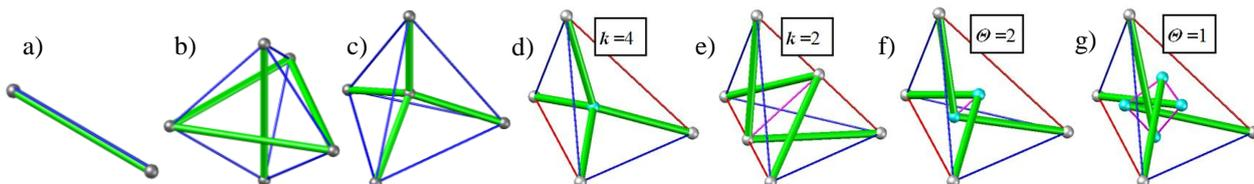
Fig. 2. Some examples of the *Class k* and *Class  $\Theta$*  tensegrity systems: a) *Class k=1*, b) *Class k=2*, c) *Class k=4*. Possible topologies of the tensegrity tetrahedron: d) by Fuller (*Class k=4*), e) by Motro (*Class k=2*), f) the *Class  $\Theta=2$*  tetrahedral cell, g) the *Class  $\Theta=1$*  tetrahedral cell.
