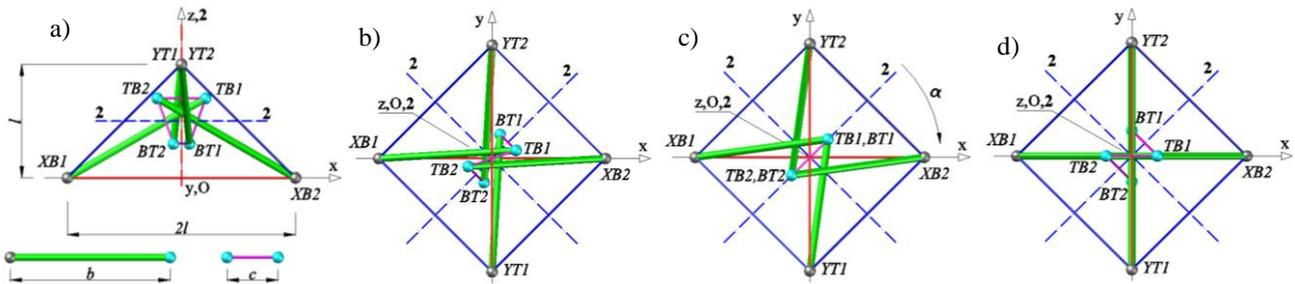
Fig. 3. Model of the Class  $\Theta = 1$  tensegrity tetrahedron: a) front view of the mother configuration, b) top view of the mother configuration, c) top view of model in the first extreme position for  $\alpha = 0^\circ$ , d) top view of model in the second extreme position for  $\alpha = 45^\circ$ .
