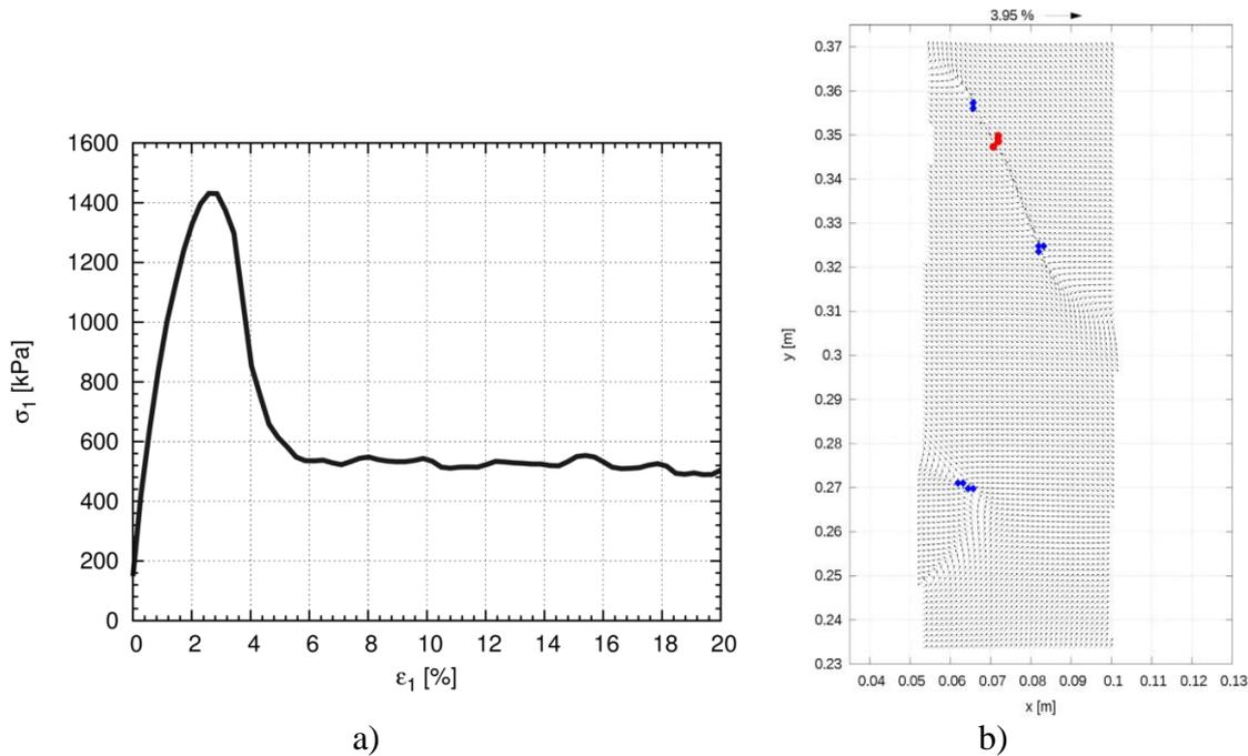
Figure 1: DEM results for plane strain compression with initially dense sand (simulated as clusters of spheres): a) vertical normal stress  $\sigma_l$  versus vertical normal strain  $\epsilon_l$  and b) distribution of single vortices and anti-vortices in normalized displacement fluctuation vector field for vertical normal strain  $\epsilon_l=3.95\%$  (red circle - left-handed vortex, blue circle - anti-vortex)
