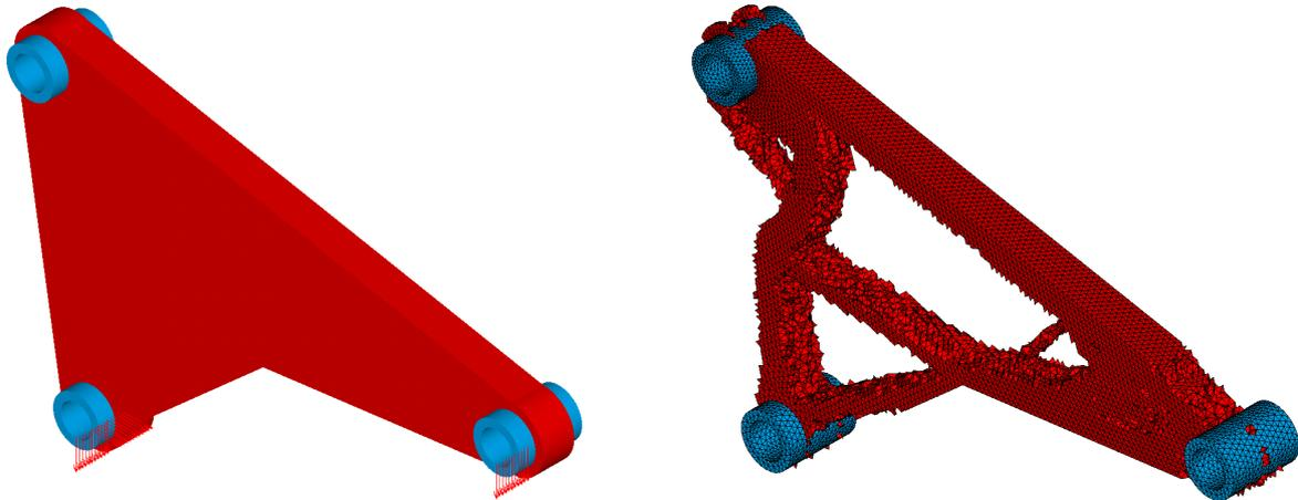
**Figure 1.** Initial structure (left), obtained topology (right)
