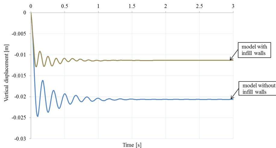
Figure 1. Time-vertical displacement curves: model with infill walls vs. model without infill walls.
