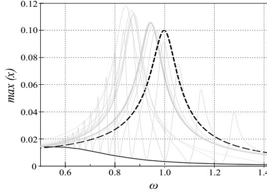
**Figure 2.** FRCs of the base oscillator with linear stiffness. The black dashed line corresponds to the FRC of system without TMD, gray lines show the FRCs for system with TMD for different  $I_D$  values while the solid black line indicates the response of the system with optimized inertance.
