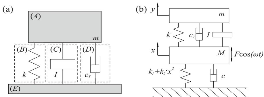
**Figure 1.** Scheme of the proposed vibration absorber (a) and the model of the investigated system (b) with notation of system's parameters.
