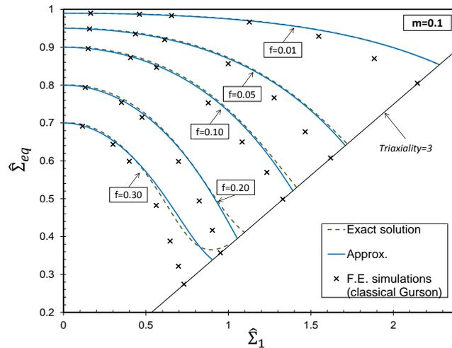
**Figure 1.** Comparison of model, numerical finite element and exact  $\hat{\Sigma}_{eq} - \hat{\Sigma}_1$  results considering the approach for porosities  $f = 0.01, 0.05, 0.1, 0.2, 0.3$  and a strain rate sensitivity parameter  $m = 0.1$ .
