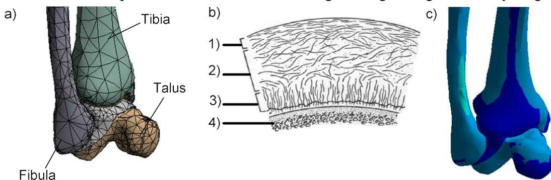
Figure 1. The upper ankle FEM model. a) Model of bones, b) The layers of articular cartilage: 1-external layer, 2-middle layer, 3-internal layer, 4- bone, c) The map of stresses on the bones
