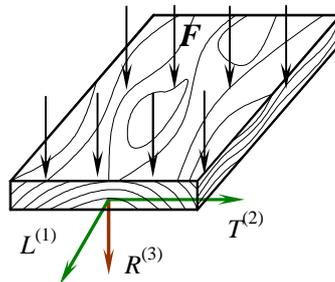
Fig. 1. Orientation of wood fibres (anisotropy):  $F$  – load,  $L$  – longitudinal direction, parallel to fibres, and two directions perpendicular to fibres:  $R$  – radial and  $T$  – tangent
