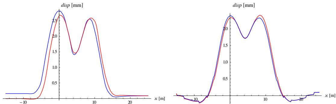
Figure 1. Vertical displacement of the shell key point during two passages of the locomotive – comparison of the in situ test results (left) and numerical simulation (right)
