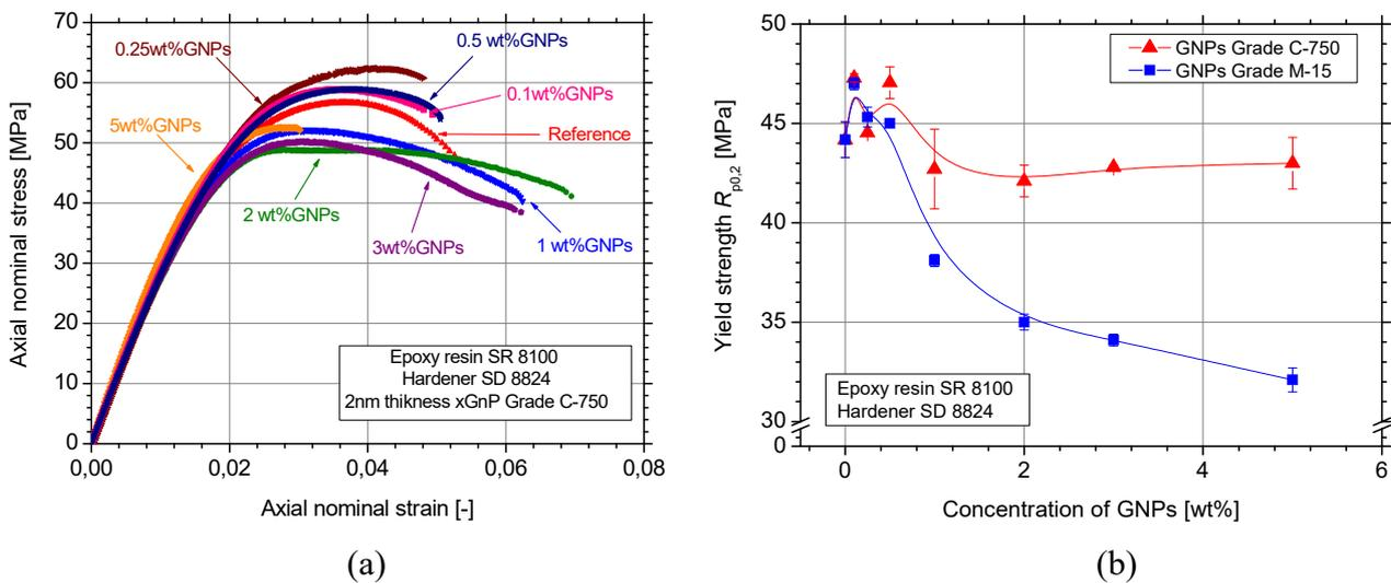
Figure 1. (a) Typical tensile flow curves of nano-reinforced resins and (b) evaluated yield stress  $R_{p0.2\%}$  of the specimens for different reinforcing concentrations.
