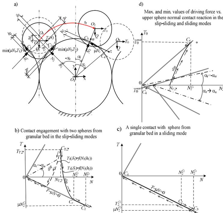
Figure 1 Sphere contact interaction with the regularly packed granular bed: evolution of contact tractions
