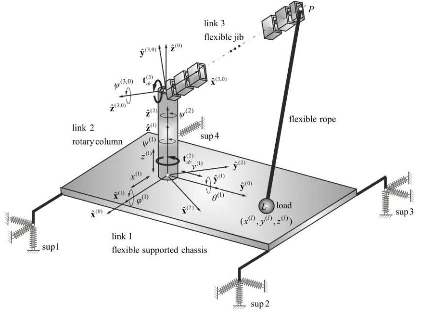
Fig. 1. Truck-crane model
