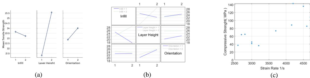
Figure 1: (a) main effect plot, (b) interaction plot for build parameters, (c) strain rate vs compressive strength of samples.
