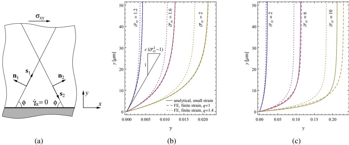
**Figure 1.** Boundary layer evolving under shear of a constrained half-space: (a) schematic description of the problem, and profiles of accumulated slip  $\gamma$  at (b) small and (c) moderate strains.
