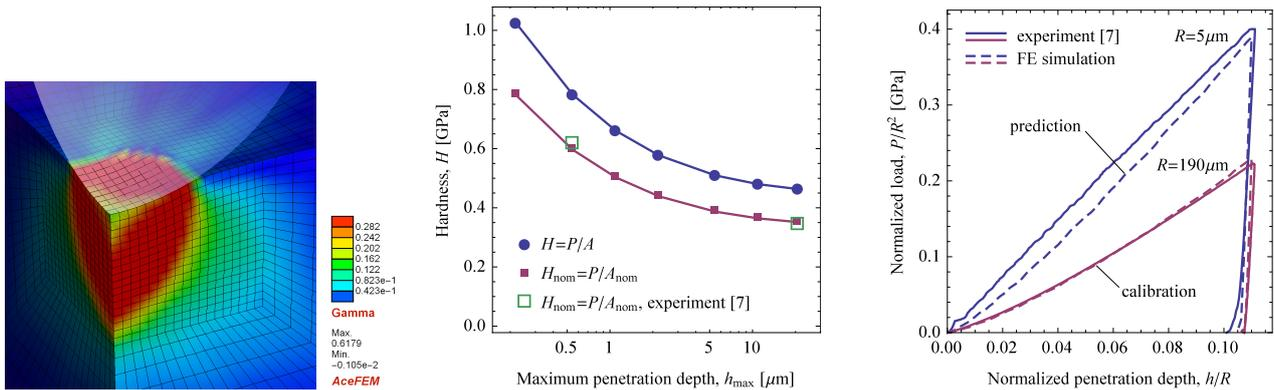
**Figure 2.** FE simulation of spherical indentation of (001)-oriented Cu single crystal: accumulated total plastic slip (left), dependence of hardness on the maximum penetration depth at fixed ratio  $h_{\text{max}}/R = 0.11$  (middle), and normalized size-dependent load–penetration depth curves (right).
