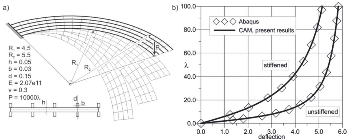
Figure 1. Stiffened quarter-ring cantilever a) geometry, material and load parameters, deformation b) load factor-deflection curves.
