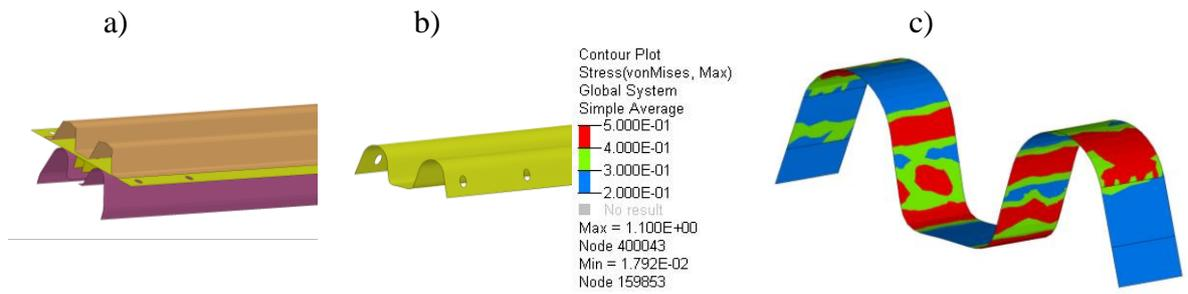
Fig.2. Simulation of a forming process: a) initial shape of the plate and stamps, b) plate in the final stage, c) reduced stress in the final stage
