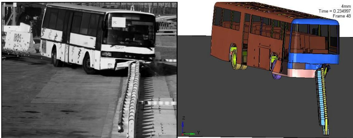
Fig.4. Deformation of bus and barrier in the experimental test and numerical simulation
