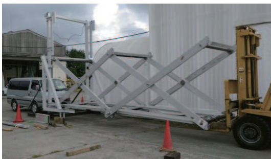
Figure 1. A two-unit experimental Mobile Bridge.
