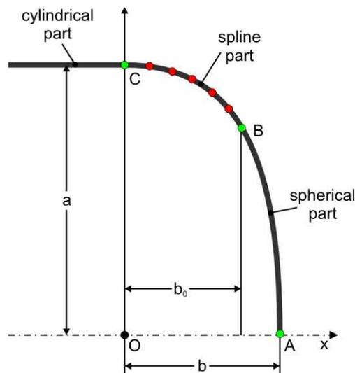
Fig. 1. The geometry of the vessel
