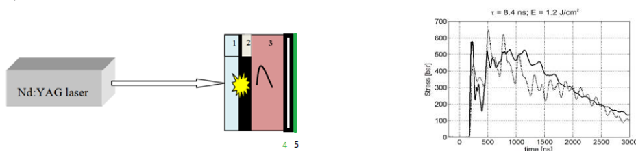
Fig. 1. A- Experimental scheme for testing dynamic hardness and adhesion of thin films. B- Comparison of calculated (- -) and experimental (--) profile of pressure of shock wave.
