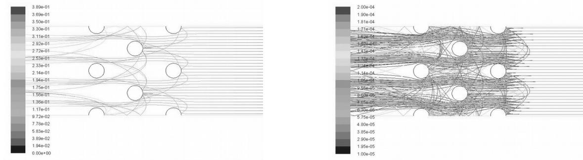
Figure 2. Solid particles’ tracks in case of their velocity of 3 m/s and uniform (100 μm-upper) or size distribution (down)
