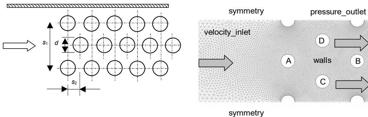
Figure 1. Staggered arrangement of U-tube recuperators and boundary conditions with mesh used in numerical simulations
