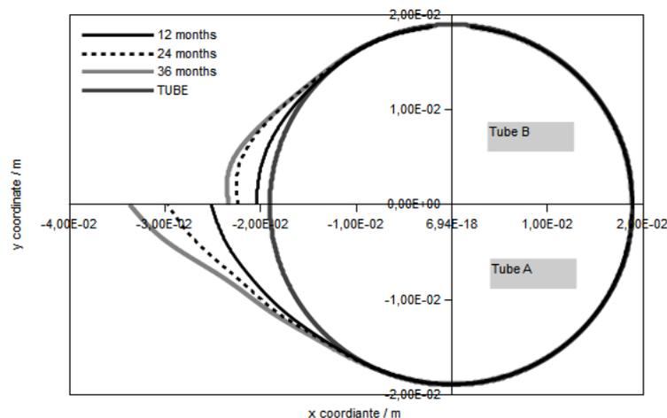
Figure 3. Shape of deposits on tubes A and B (velocity is 5 m/s, solid particles mass flow is 0,17 mg/s)
